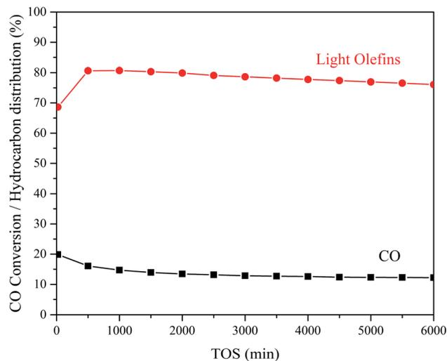
Fig. 7 Stability test of the catalytic performance for the STO reaction over  $\text{ZnCrO}_x + \text{SAPO-18}(0.048)$  bifunctional catalyst. Reduction condition: 583 K, atmospheric  $\text{H}_2$ , GHSV =  $6000 \text{ mL g}^{-1} \text{ h}^{-1}$ . Reaction condition: 653 K, 1.0 MPa, GHSV =  $6000 \text{ mL g}^{-1} \text{ h}^{-1}$ , TOS = 6000 min,  $\text{H}_2/\text{CO}/\text{N}_2 = 6/3/1$ , OX/ZEO = 2.
