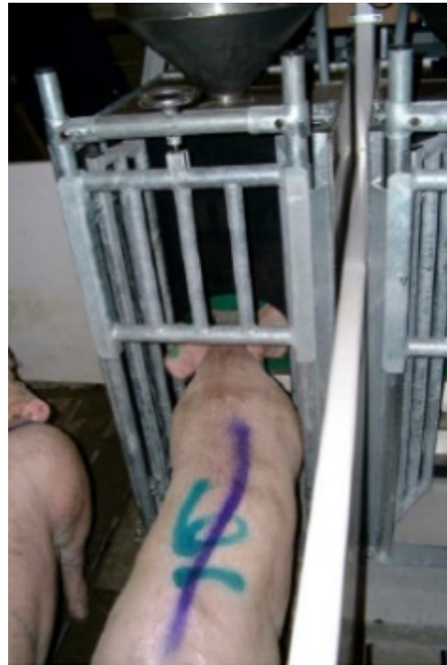
Figure 2. IVOG—A station for individual feed intake recording in group housing (Instentec B.V., Marknesse, the Netherlands) used in the studies of De Haer and Merks, [12], De Haer et al. [10], De Haer and de Vries, [8], Georgsson and Svendsen, [47,48], Rauw et al. [4], and Fernández et al. [26] (Source: [ www.insentec.eu ], accessed on 5 April 2022).
