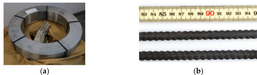
Figure 1. Iron-based shape memory alloy in the form of: (a) strips, reprinted with permission from ref. [18]. Copyright 2018 Elsevier; (b) bars, reprinted with permission from ref. [20]. Copyright 2016 Elsevier.
