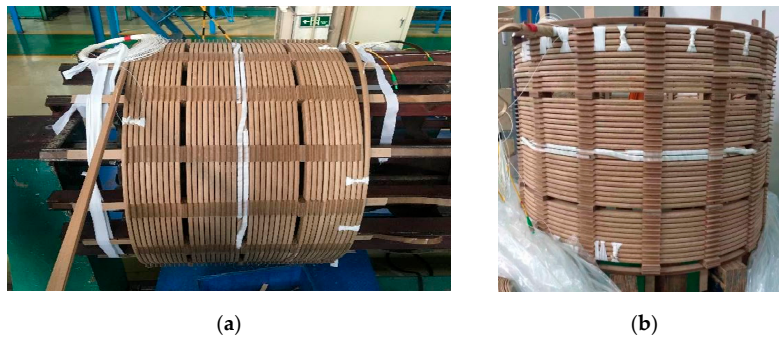
Figure 10. (a) The installation of fibre-optic composite transformer winding model and (b) the completed transformer winding model.
