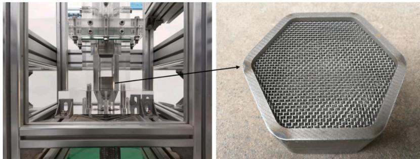
Fig. 4. The multi-layer screen filter plug in the bottom nozzle.
