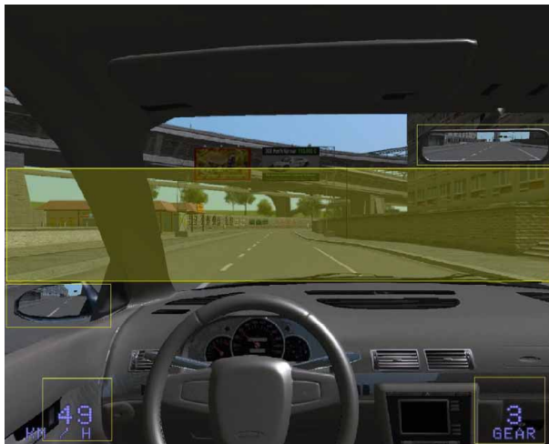
Figure 3. Illustration of the visual area of interest (roadway) highlighted in yellow. Screen dimensions: 1280 \times 1024 pixels ( 41.9 \times 33.4 cm; 38.5 \times 31.1 deg). Interest area dimensions: 1280 \times 266 pixels ( 41.9 \times 8.7 cm; 38.5 \times 8.3 deg).
