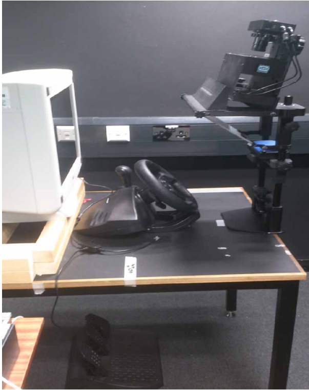
Figure 2. Apparatus set up of monitor (left), steering wheel, pedals and eye tracker.
