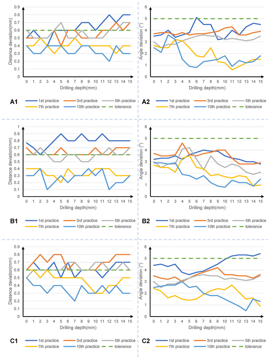
Figure 3 Influence of learning times on the positioning accuracy of different drilling depths under the guidance of dynamic navigation. (A1, A2) Distance and angle deviation for operator 1, (B1, B2) Distance and angle deviation for operator 2, (C1, C2) Distance and angle deviation for operator 3, (D1, D2) Distance and angle deviation for operator 4, (E1, E2) Distance and angle deviation for operator 5, (F1, F2) Distance and angle deviation for operator 6.
