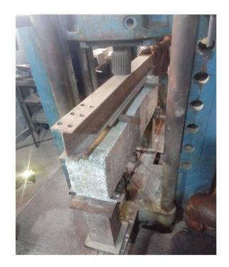
Figure 8. Testing of a beam using an ultimate testing machine.
