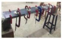
(h) Compressing the composite plate by clamps.
