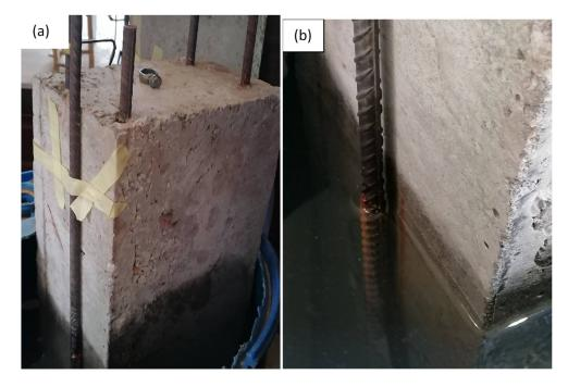
Figure 12. Evidence of corrosion on beams: (a) At early stage; (b) at maturity.
