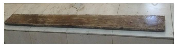
Figure 2. Fabricated bamboo laminate.
