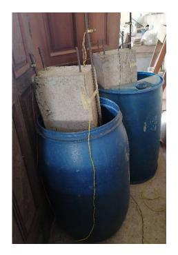
Figure 5. Simulated corrosion set-up in the laboratory.
