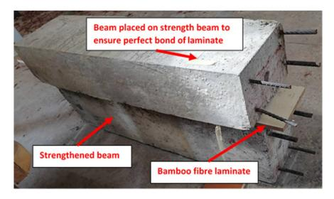
Figure 6. Bonding of bamboo laminate to the surface of the corroded beam.
