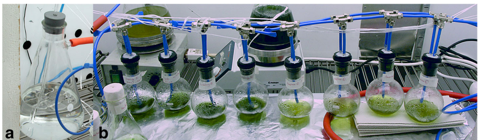
Fig. 1 The vacuum line set-up where the flowing gas is first saturated with water vapor ( left ) and then lead into the culture bottles. The air flow is regulated with a rheostat and the pressure inside the whole closed system by a pressure gauge, and a vacuum pump (vacuubrand)
