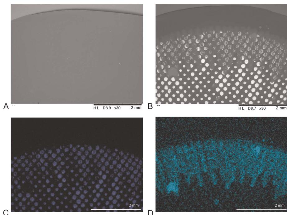
**FIG. 5.** Scanning electron microscopy views and mapping analysis of JOY POP RICH. (A) The surface of the anterior side is smooth. (B) Colorants are deposited on the posterior side. (C) Blue shows the distribution of iron. (D) Light blue shows the distribution of chlorine.
