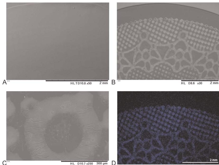
**FIG. 2.** Scanning electron microscopy views and mapping analysis of EYE COFFRET 1-DAY UV. (A) The surface of the eyelid side is smooth. (B) The print design is apparent on the posterior side, and the pattern is uniform. (C) A coated thin layer is wrinkled. (D) Blue shows the distribution of chlorine.
