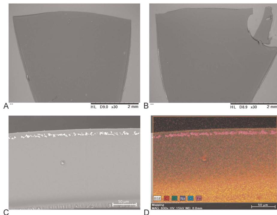
**FIG. 1.** Scanning electron microscopy views and energy-dispersive x-ray mapping analysis of 1-DAY ACUVUE DEFINE. (A) The surface of the eyelid side is smooth. (B) The surface of the corneal side is also smooth. (C) The cross section reveals that the colorants are located to a depth of 8 to 14  $\mu\text{m}$  from the eyelid side of the lens. (D) The main component of the colorants is iron.
