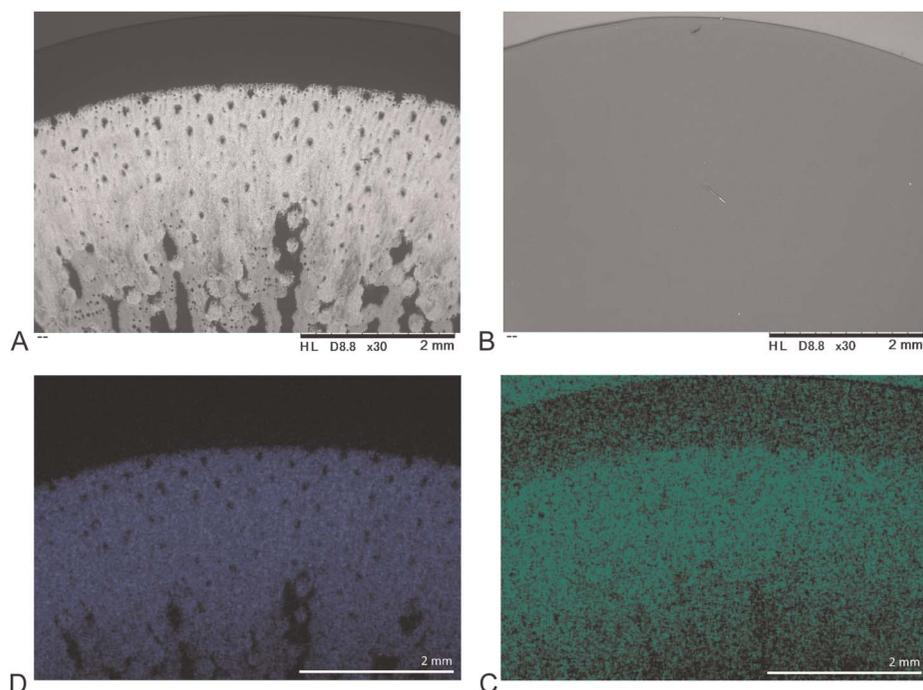
**FIG. 4.** Scanning electron microscopy images and mapping analysis of TUTTI VANITY RICH. (A) Colorants are deposited on the anterior side. (B) The surface of the posterior side is smooth. (C) Blue shows the distribution of iron. (D) Green shows the distribution of oxygen.
