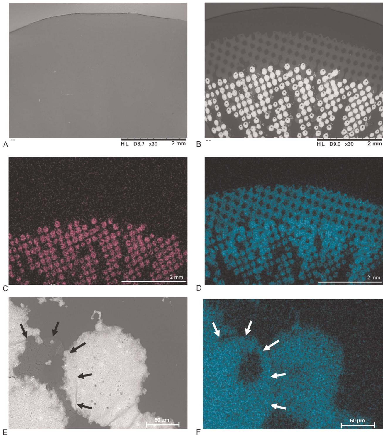
**FIG. 3.** Scanning electron microscopy views and mapping analysis of EVER COLOR 1-DAY NATURAL. (A) The surface of the anterior side is smooth. (B) Colorants are deposited on the posterior side. (C) Purple shows the distribution of titanium. (D) Light blue shows the distribution of chlorine. (E) Black arrows show exuded chlorine in high magnification. (F) White arrows show exuded chlorine.
