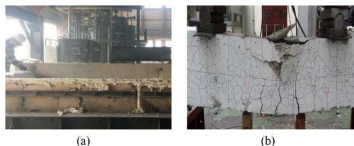
Figure 6. (a) Fire experiments to construct the database and (b) the concrete structures after the fire.
