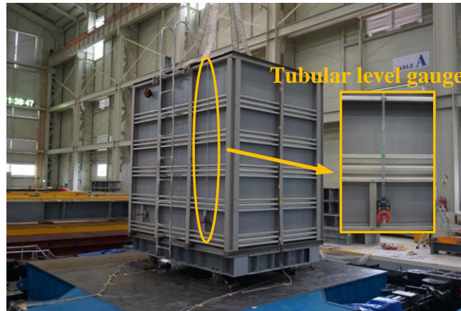
Figure 3. Specimen installed on the shaking table.
