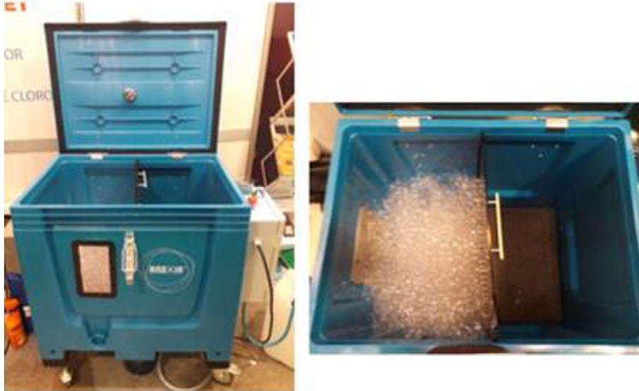
Figure 13: Foam system for piglets (Source: Anoxia B.V.) the space in the box can be adjusted to group or animal size
