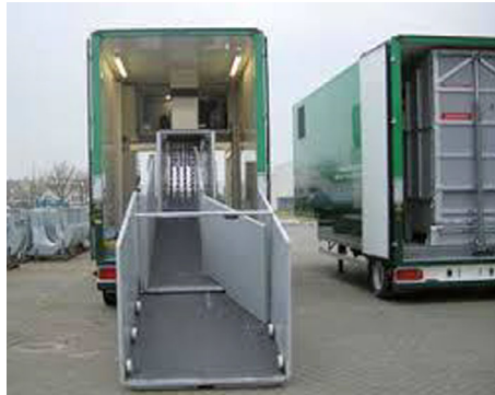
Figure 5: Swine mobile electrocution unit for the mass depopulation of swine (courtesy of Marien Gerritzen)
