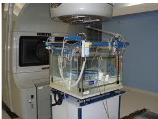
Figure 4: Varian Linac and water phantom
