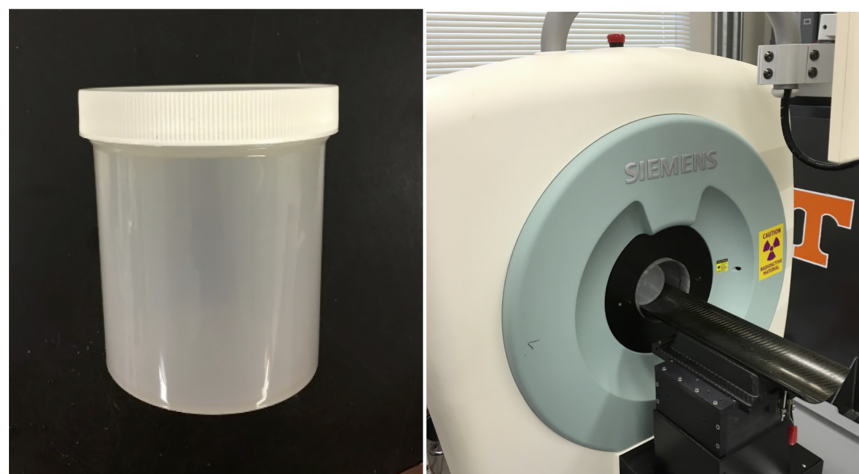
Fig 2. Photographs of experimental equipment. (Left) 500 mL bottle used in cell tracking experiment. (Right) Photograph of bottle placed into bore of PET scanner.
