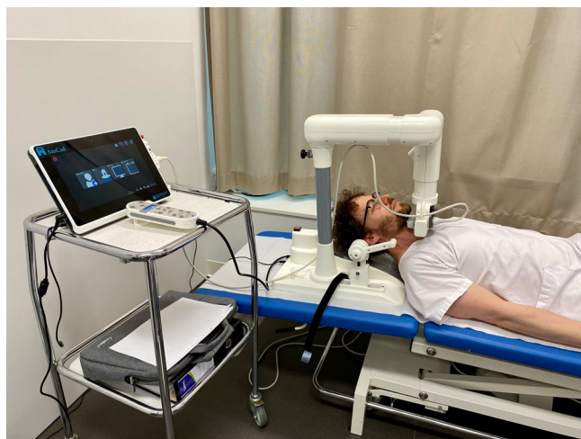
Figure 1. Ultrasonography system with a robotic probe positioning and laser alignment tool to ensure standardized scanning of the upper airway (AmCad BioMed Corporation).
