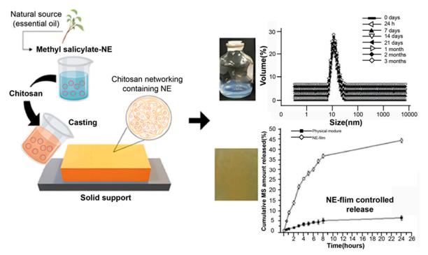
**Figure 3.** Schematic diagram of the process of nanoemulsions (NE)-film and the size and PDI analysis of formulation for three months after ultrasonication process and the release effect compared with a physical mixture for 24 h [82]. Reproduced with permission from Talita Nascimento daSilva, International Journal of Biological Macromolecules; published by Elsevier, 2020.
