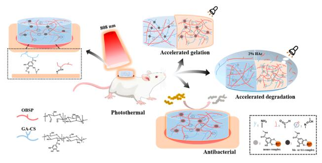
**Figure 2.** A schematic diagram of the dual network polysaccharide hydrogel and photothermal effect accelerated the gelation and degradation rate of the hydrogel and gallic acid with Fe<sup>3+</sup> showed good antibacterial properties. OBSP: oxidized *Bletilla striata* polysaccharide; GA-CS: gallic acid grafted chitosan [66]. Reproduced with permission from Chonghao Chen, Carbohydrate Polymers; published by Elsevier, 2021.
