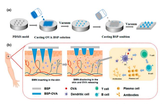
**Figure 4.** Schematic diagram of the preparation process and ovalbumin (OVA) delivery condition. (a) Two-step preparation of *Bletilla striata* polysaccharide (BSP) microneedle (MN) (BMN). (b) Transdermal drug delivery of the OVA-loaded BMN system and the release of the drug can be triggered by the dissolving of BSP in the skin interstitial fluid [97]. Reproduced with permission from Ping Zhou, International Journal of Biological Macromolecules; published by Elsevier, 2022.
