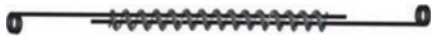
FIGURE 2: Insert straight parts of both guide wires through both sides of lumen opening of open-coil spring, and pass them through the entire lumen towards each other (in opposite directions).
