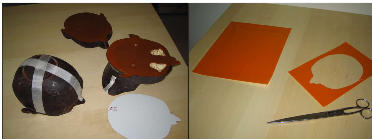
Figure 1. The anatomical head phantom and the Gafchromic® film cut to fit between the different layers of the phantom.
