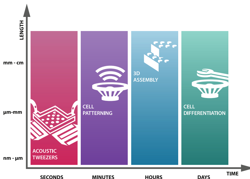
Fig. 1. Use of acoustic manipulation on different length and time scales. Acoustic manipulation or sound patterning can be applied over seconds, minutes, or even hours or days to perform long-term stimulation. On the length scale, nano- or microparticles can be manipulated by acoustic tweezers, individual cells can be patterned within 2 or 2.5 dimensions, whereas 3D constructs were prepared by cell spheroid assembly.
