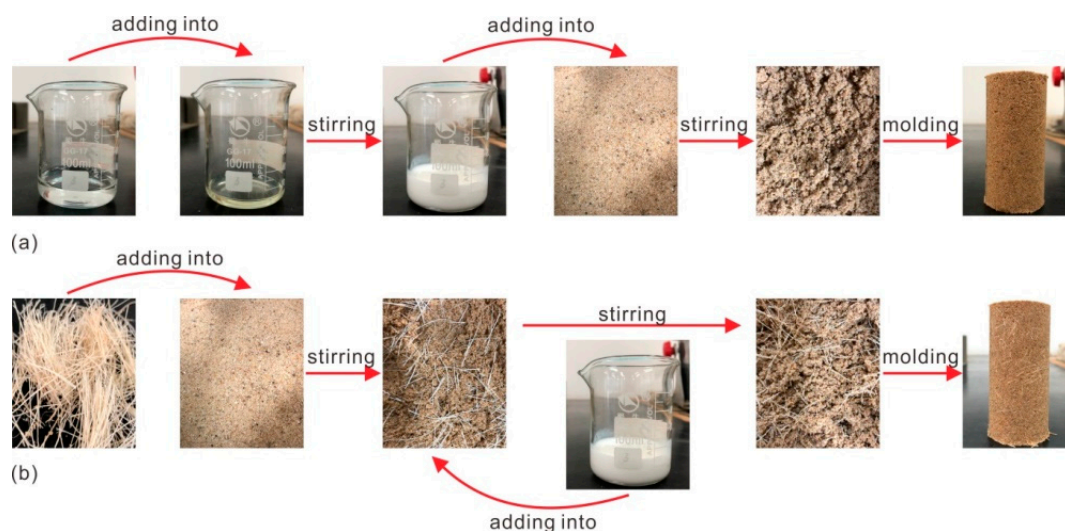
Figure 4. The diagram of the composite specimen fabrication: (a) OPSS and (b) OPSS with fiber.
