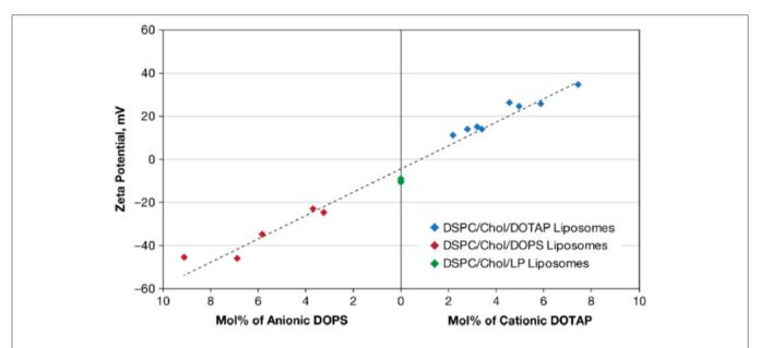
**FIGURE 6** | Zeta potentials in 0.01 mol/L NaCl (pH 7.4–7.7) of cholesterol (Chol), 1,2-distearoylsn-glycero-3-phosphocholine (DSPC) liposomes. Liposomes were made positively-charged with varying mol% of DOTAP (1,2-dioleoyl-3-trimethylammonium-propane) or negatively-charged with DOPS (1,2-dioleoyl-sn-glycero-3-phospho-L-serine). Liposomes indicated as DSPC/Chol/LP liposomes were prepared with lipid-PEG (poly-ethylene glycol) added (Smith et al., 2017) (with permission of Springer).
