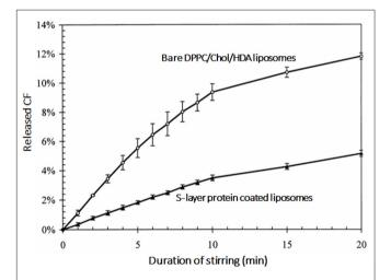
FIGURE 7 | Release of fluorescent carboxyfluoresceine (CF) as an indication of the lipid bilayer stability of dipalmitoylphosphatidylcholine (DPPC), cholesterol and hexadecylamine (HDA) liposomes as a function of stirring time in the absence and presence of a bacterial S-layer coating on the liposomes (Mader et al., 1999) (with permission of Elsevier).
