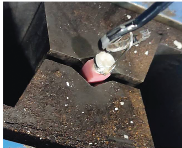
Fig. 3: Stainless steel band cemented over zirconia crown and mounted over universal testing machine
