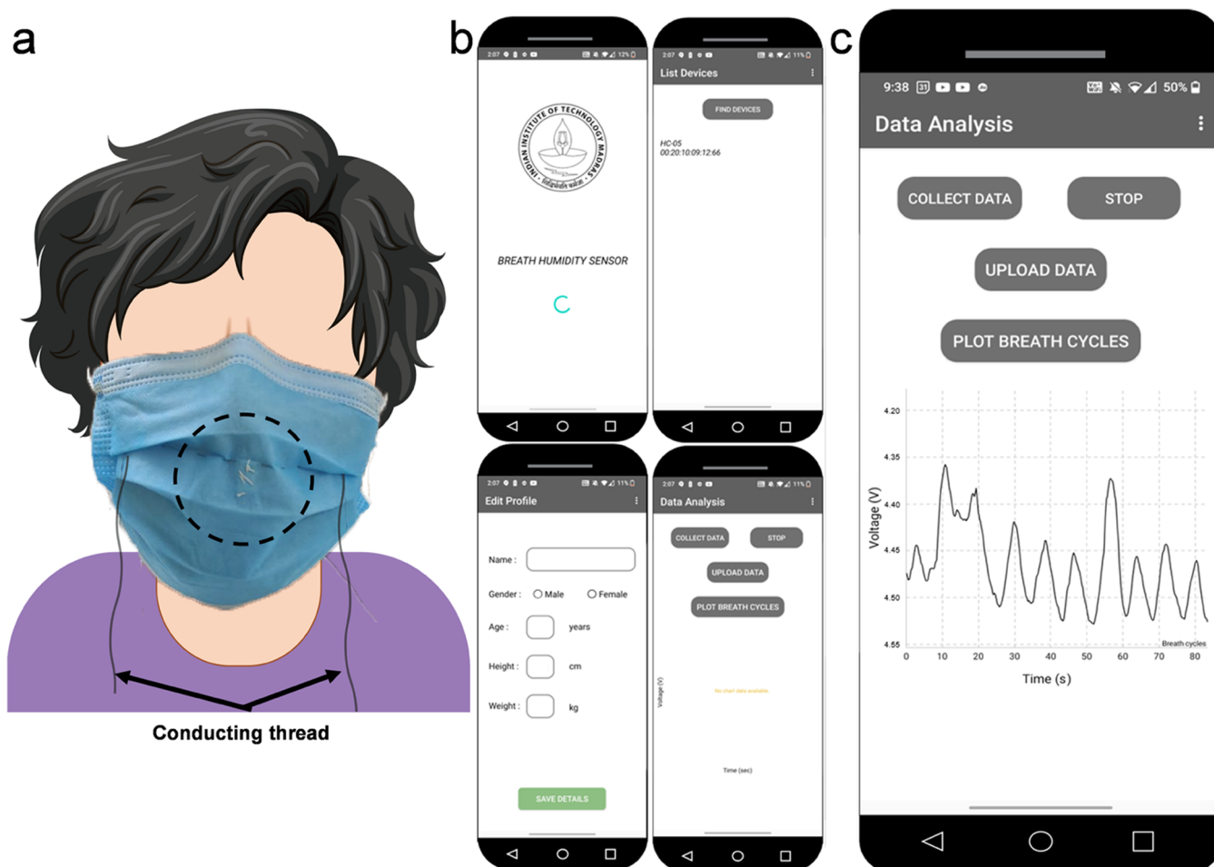
Figure 5. (a) Photograph of a volunteer wearing the mask. (b) Screen grabs of the Android application designed to monitor the breathing pattern. (c) Breathing patterns of a volunteer recorded using the mobile application depicting normal breathing.
