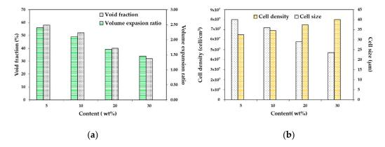
**Figure 11.** Effect of jute fiber content on the foam microstructure of the PLA/jute fiber biocomposites; (a) void fraction and volume expansion ratio and (b) cell size and cell density. Data taken from Zafar et al. [128].
