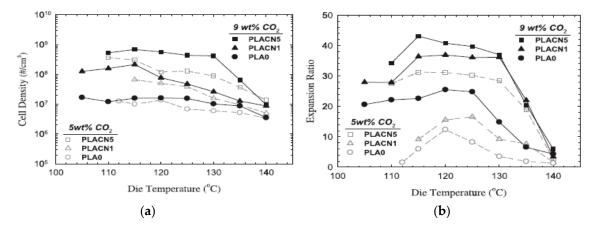
**Figure 32.** Comparison of (a) cell density and (b) expansion ratio of foams obtained at various die temperatures with 5 and 9 wt% CO<sub>2</sub> from neat PLA (PLA0) and PLA with 1 wt% (PLACN1) and 5 wt% (PLACN5) of Cloisite 30. Reprinted from Keshtkar et al. [151]. Copyright (2020), with permission from Elsevier.
