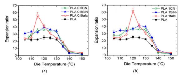
**Figure 33.** Expansion ratio of the foamed PLA and PLA/Clay, PLA/Silica and PLA/Talc composites at various die temperatures (a) Content of 0.5 wt% and (b) Content of 1 wt%. Reprinted from Nofar [113]. Copyright (2020), with permission from Elsevier.
