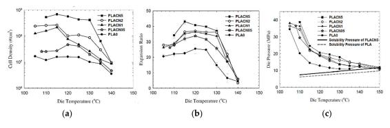
**Figure 30.** (a) Cell density and (b) expansion ratio of PLA & PLA/Cloisite 30 (PLACN) foams processed at various die temperatures, and (c) die pressure and solubility pressure at various die temperatures. Reprinted from Keshtkar et al. [151]. Copyright (2020), with permission from Elsevier.
