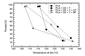
**Figure 29.** Effect of formulation and mixer and die temperatures on the porosity of PLA foams extruded at 8% of CO<sub>2</sub>. Reprinted from Bocz et al. [150] with the permission of Express Polymer Letters.
