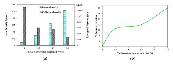
**Figure 15.** Foam characterization of PLA/wood flour composite foams: (a) Foam density and cell density, and (b) expansion ratio as a function of CE content. Data taken from Wang et al. [130].
