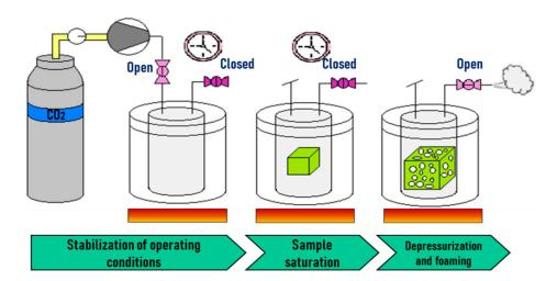
Figure 8. Pressure-induced foaming process. Adapted from Standau et al. [132].
