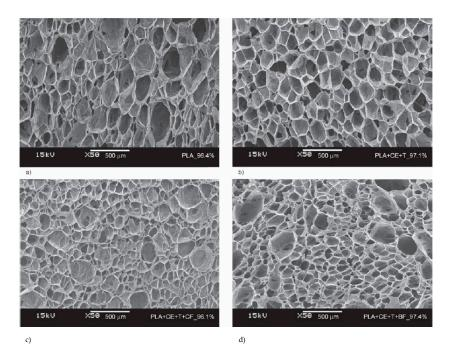
**Figure 36.** SEM micrographs of the cell morphologies obtained for highly expanded ( $\varepsilon > 95\%$ ) PLA foams. (a) PLA, (b) PLA + CE + T, (c) PLA + CE + T + CF, and (d) PLA + CE + T + BF. Reprinted from Bocz et al. [150] with permission from Express Polymer Letters.
