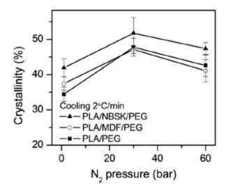
**Figure 21.** Degree of crystallinity of the PLA composites at a cooling rate of 2  $^{\circ}$ C/min under various N<sub>2</sub> pressures. Reprinted from Ding et al. [138]. Copyright (2020), with permission from Elsevier.
