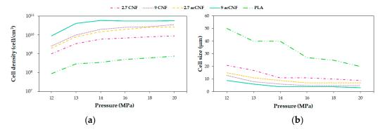
**Figure 14.** Effect of variations in pressure on the (a) average cell diameter and (b) cell density of the neat PLA and PLA/aCNFs nanocomposite foams. Data taken from Dlouhá et al. [126].
