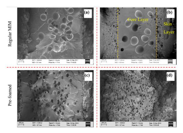
**Figure 27.** Cellular structures of (100× magnification): (a) neat PLA foam without pre-foaming, (b) PLA/clay foam without pre-foaming, (c) neat PLA foam with pre-foaming, and (d) PLA/clay foam with pre-foaming. Reprinted from Zhao et al. [90]. Copyright (2020) American Chemical Society.
