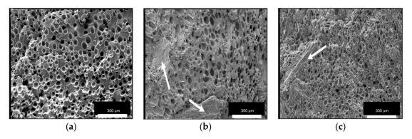
**Figure 23.** Scanning electron microscopy (SEM) image of foamed samples: (a) virgin PLA, (b) PLA/willow-fiber (80/20), and (c) PLA/willow-fiber (70/30). Reprinted from Zafar et al. [137]. With permission from Express Polymer Letters.
