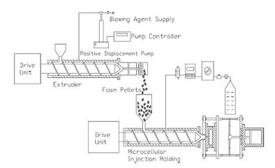
**Figure 26.** Schematic of microcellular injection molding combined with the pre-foaming extrusion process developed by Zhao et al. Reprinted from Zhao et al. [90]. Copyright (2020) American Chemical Society.
