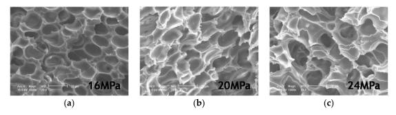
**Figure 10.** Effect of pressure on cell morphology of PLA/silk foams (7 wt%, 155 °C) at (a) 16 MPa, (b) 20 MPa, and (c) 24 MPa. Reprinted from Kang et al. [129]. Copyright © 2020 WILEY-VCH Verlag GmbH & Co. KGaA, Weinheim.
