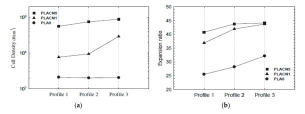
**Figure 31.** (a) Cell density and (b) expansion ratio of foams obtained by varying temperature profiles in the second extruder of tandem line foaming extrusion system from neat PLA (PLA0) and PLA with 1 wt% (PLACN1) and 5 wt% (PLACN5) of Cloisite 30. Reprinted from Keshtkar et al. [151]. Copyright (2020), with permission from Elsevier.
