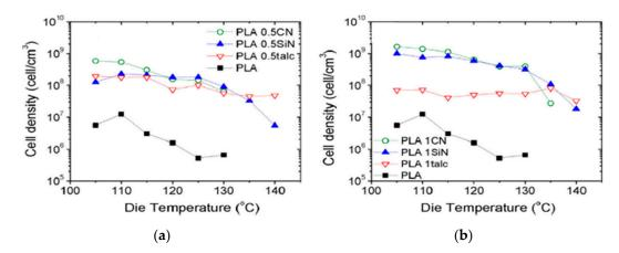
**Figure 34.** The cell density of foamed PLA and PLA/clay, PLA/silica, and PLA/talc composites at various die temperatures, (a) content of 0.5 wt% and (b) content of 1 wt%. Reprinted from Nofar [113]. Copyright (2020), with permission from Elsevier.
