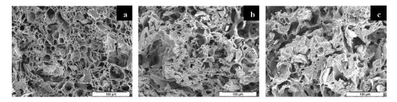
**Figure 37.** Effect of rheology modifier content on cell morphology of foamed PLA samples containing 20 wt% wood flour: (a) 2 wt%, (b) 4 wt%, and (c) 6 wt% E-43. Reprinted from Matuana and Díaz [155]. Copyright (2020) American Chemical Society.
