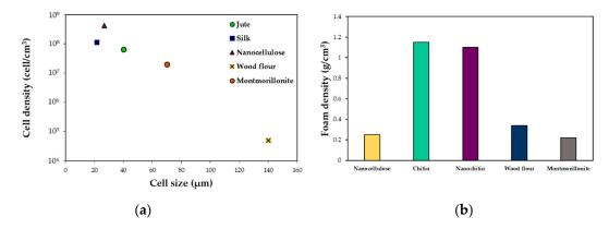
**Figure 17.** (a) Cell density and cell size for different fillers at 5 wt% content in PLA and (b) foam density for different fillers between 3 and 5 wt% contents in PLA. Data taken from Zafar t al. [128], Kang et al. [129], Cho et al. [125], Neagu et al. [127], and Ema et al. [131].
