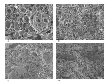
**Figure 4.** Effect of wood fiber content on the cellular structures of PLA: (a) 10 wt%, (b) 20 wt%, (c) 30 wt%, and (d) 40 wt%, saturation pressure 2.76 MPa for 4 days, magnification (100×). Reprinted from Matuana and Faruk with permission from Express Polymer Letters [123].
