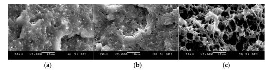
**Figure 3.** PLA/CNFs (1 wt%) foams micrographs at (a) 100 °C, (b) 110 °C, and (c) 120 °C. Reprinted from Ding [120].
