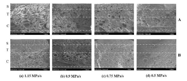
**Figure 19.** Representative SEM micrographs of the injected foams of pure PLA (**A**) and PLA/nanoclays (**B**) with four different dropping pressure speeds (1.15, 0.9, 0.75, and 0.5 MPa/s). Reprinted from Xie et al. [136].
