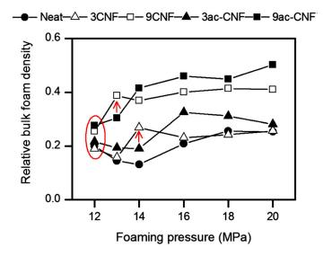
**Figure 13.** Variations of the relative bulk foam density of PLA foams as functions of foaming pressure. Arrows indicate the foaming pressure at which the relative bulk foam density increases suddenly for the CNFs composites. Reprinted from Dlouhá et al. [126]. Permission conveyed through Copyright Clearance Center, Inc.
