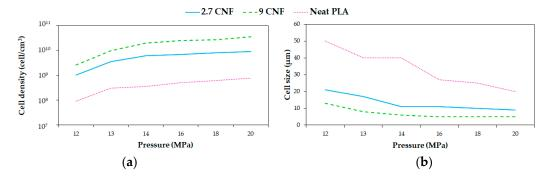
**Figure 9.** Effect of pressure in (**a**) cell density and (**b**) cell size of PLA/CNFs foams. Data taken from Dlouhá et al. [126].
