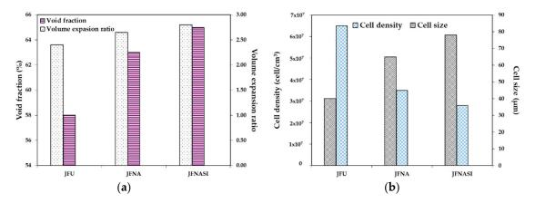
**Figure 12.** Effect of jute fiber surface treatment on the foam microstructure of the PLA/jute fiber biocomposites: (a) void fraction and expansion ratio (b) cell size and cell density. Data taken from Zafar et al. [128].
