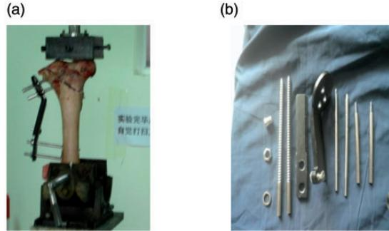
**Figure 2.** Slide-poking external fixator. (a) View of external fixator after assembly and fixation. (b) Parts of external fixator.
