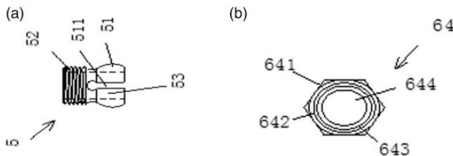
**Figure 4.** Universal joint and nut. (a) Universal joint. 51–Ball. 52–Cylindrical portion. 53–Center hole. 511–Radial groove. (b) Nut. 64–Joint nut. 641–Outside six-party. 642–Spherical flange. 643–Flange bore. 644–Internally threaded cap portion.
