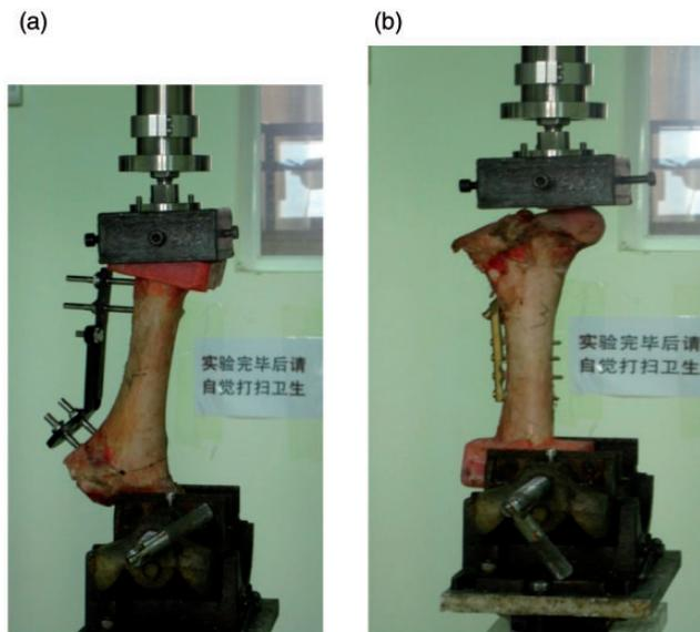
**Figure 11.** Vertical loading test. (a) External fixator. (b) Dynamic hip screw.
