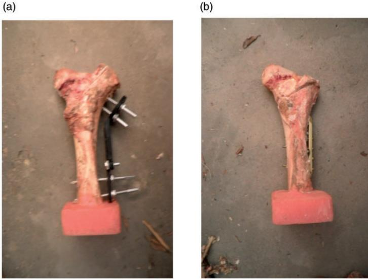
**Figure 9.** Establishment of fracture model. (a) External fixator. (b) Dynamic hip screw.
