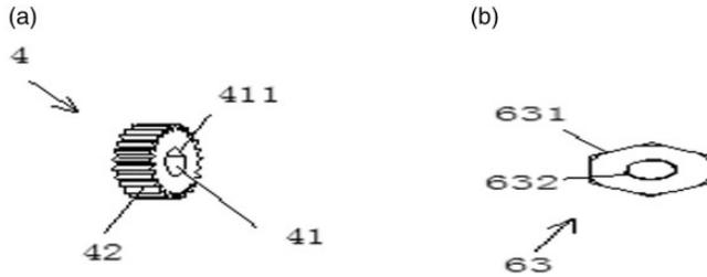
**Figure 6.** (a) 4–Shank. 41–Shaft hole. 42–Tooth pattern. 411–Platform. (b) 63–Gear. 631–Hexagon. 632–Inside thread.
