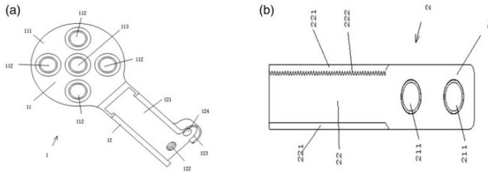
**Figure 3.** Sliding plate. (a) Head and body. 11–Head. 12–Body. 111–Ball fossa. (b) Far sheet plate. 21–Fixed part. 112, 113–Universal joint holes. 22–Bolt. 211–Bone screw hole. 114–Embossed surface. 121–Chute. 221–Gave way trough. 222–Tooth groove. 122–Hole of top cone screw. 123–Gear nest. 124–Shaft hole.
