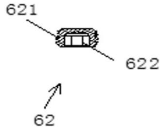
**Figure 7.** Top bolt screw setting. 621–External thread screw of top taper. 622–Hexagon socket.
