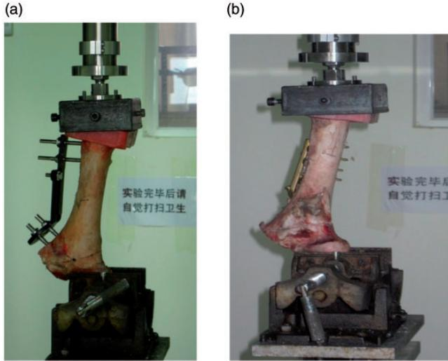
**Figure 12.** Torsional loading test. (a) External fixator. (b) Dynamic hip screw.
