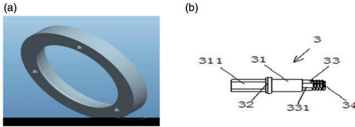
**Figure 5.** Gasket and drive shaft. (a) Point-like projections of gasket. (b) 3–Drive shaft. 31–Shaft. 32–Apron. 311–Crude. 331–Gear shaft. 34–Screw thread.
