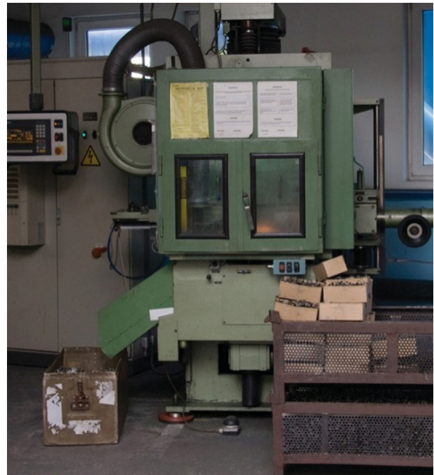
Figure 2. An overall view of the workstation for grinding spring faces.
