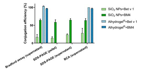
**Figure 2.** Conjugation efficiency of particulate systems. The quantitative analysis of percentage of allergen bound to  $SiO_2$  NPs and Alhydrogel<sup>®</sup> was performed by SDS-PAGE, Bradford assay and BCA assay. A 100% conjugation efficiency here represents a conjugation of the total amount of allergen taken for the experiment (160 µg/mL).
