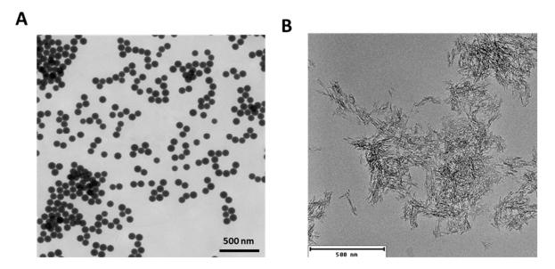
**Figure 1.** Characterization of the particulate systems by determining the morphology and primary size of particles. Transmission electron microscopy (TEM) image of synthesized SiO<sub>2</sub> NPs (**A**) and Alhydrogel<sup>®</sup> (**B**).
