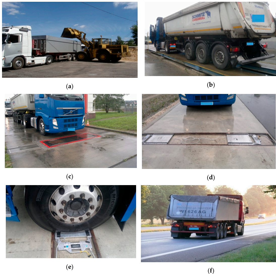
Figure 3. Preparation of reference vehicles: (a)—loading the vehicle with gravel; (b)—the measurement of GVW on a platform scale; (c)—the measurement of axle load and GVW on a low-speed scale; (d,e)—the measurement of static axle load on a static scale; (f)—weighing of the vehicle at the MS-WIM site.
