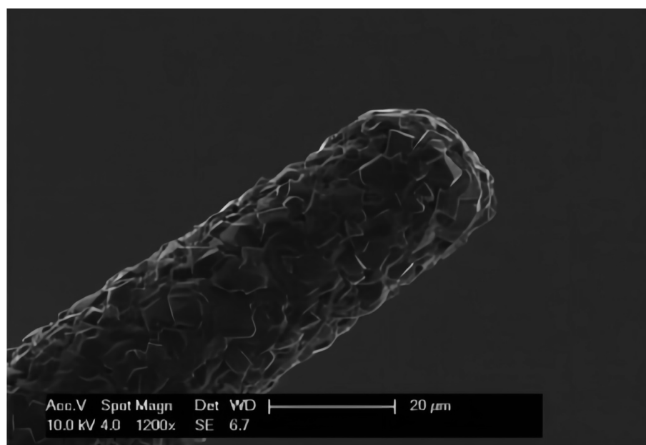
Fig. 9 SEM image of the BDD microelectrode. The image shows the tip of the needle shaped BDD microelectrode. Figure from Stéphane Fierro et al. 49 Reproduced with permission from Sci. Rep. , 2012, 2. Copyright nature Ltd (2012).
