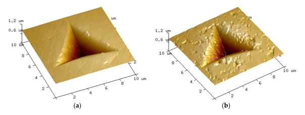
**Figure 7.** 3D AFM images of residual indents on: (a) undamaged surface (#PRIST); and (b) area of wear stripe (#SH9).
