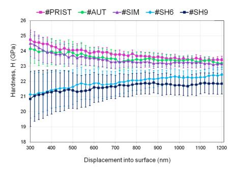
**Figure 8.** Hardness evolution as a function of penetration depth: averaged curves over the fifteen independent measurements performed on every sample.
