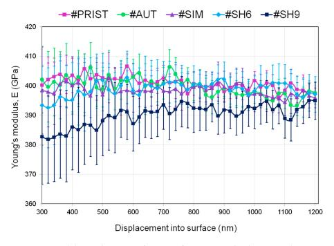
**Figure 9.** Young's modulus evolution as a function of penetration depth: averaged curves over the fifteen independent measurements performed on every sample.
