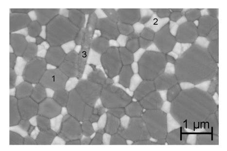
**Figure 1.** Scanning Electron Microscopy (SEM) image of a thermally etched as-received Biolox<sup>®</sup> delta implant: (1) alumina grain; (2) yttria-stabilized zirconia grain; and (3) platelet-shaped crystal of strontium aluminate.
