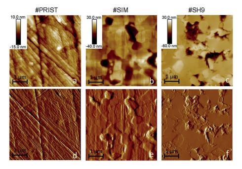
**Figure 3.** AFM height (top) and derivative (bottom) images of the control-sample #PRIST ((**a**) and (**d**)), the sample #SIM ((**b**) and (**e**)) and the sample #SH9 (wear stripe area, (**c**) and (**f**)).
