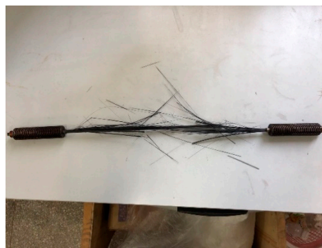
Figure 6. Fatigue failure of tendons.
