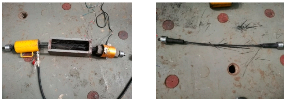
Figure 5. Failure mode of CFRP tendons.
