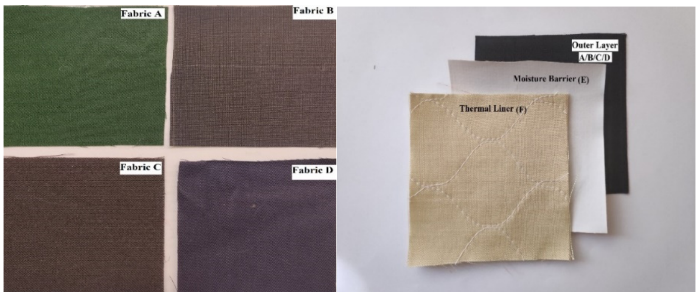
Figure 1. Fabric A, B, C, D, and an arrangement of a three-layered fabric system.
