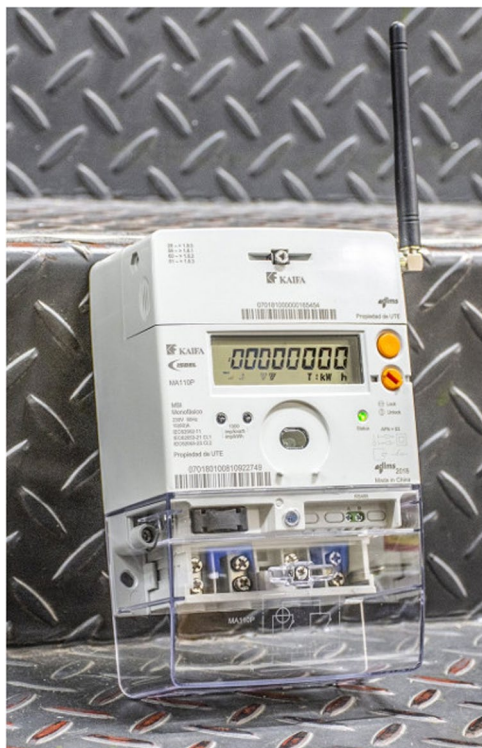
Fig. 2 Smart meter Kaifa, model MA110P, installed by the Uruguayan electricity company, UTE (image by UTE, https://portal.ute.com.uy/medicion-inteligente ).
