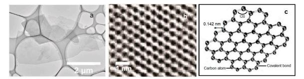
**Figure 12.** Morphological characterization of graphene structure. (a) Transmission electron microscopy image at low magnification showing several overlapping graphene flakes [43], (b) spherical aberration-corrected high-resolution transmission electron microscopy image of the honeycomb structure of a graphene single-layer sheet [44], (c) Single graphene nanosheet [45]. Partially reprinted with the permission of the authors [43–45].
