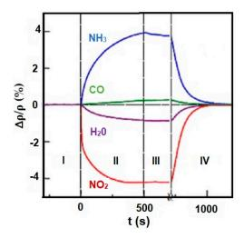
**Figure 10.** Changes in resistivity ( $\rho$ ) of graphene exposed to NH<sub>3</sub>, CO, H<sub>2</sub>O, and NO<sub>2</sub>. Region I—the device in a vacuum before its exposure, II—exposure to a diluted chemical, III—the erasure of the experimental setup, IV—annealing (150 °C). Reprinted with permission [41].
