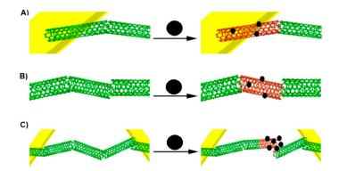
**Figure 6.** Three ways of CNT conductance change by analytes. **(A)** Modulation of the Schottky barrier at CNT-electrode junctions, **(B)** charge transfer between the analyte and CNT, **(C)** increasing the CNT–CNT junction distance by intercalation of the CNT network. Adapted from [26,29]. Black sphere-analyte, green cloud—current allowed, red cloud—current inhibited.
