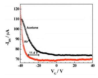
**Figure 5.** Transfer characteristic of iron tetraphenyl porphyrin-CNT in the presence of air and acetone.  $V_G$ —gate voltage,  $I_{DS}$ —the source-drain current. Reprinted with the authors' permission [21]. The amount of voltage shift has been marked.
