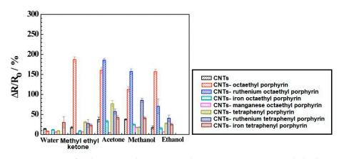
**Figure 3.** Comparison of carbon nanotubes (CNT) and various CNT-porphyrins hybrids responses towards different gases and water. Reprinted with the authors' permission [21].
