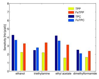
**Figure 11.** Sensitivity of free-base porphyrin (TPP) and porphyrin with iron (FeTPP) in comparison to analog porphyrin (TPC) and analog porphyrin with iron (FeTPC). Units of Hz per relative concentration ( $p/p_0$ ). Partially reprinted with permission [34].
