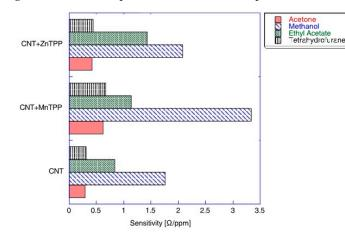
**Figure 4.** Sensitivity of the sensors composed of Mn-tetraphenylporphyrin-CNT, Zn-tetraphenylporphyrin-CNT hybrids, and CNT towards four vapors. The maximum sensitivity corresponds to the sensor sensitivity at low concentrations. Reprinted with the authors' permission [25].
