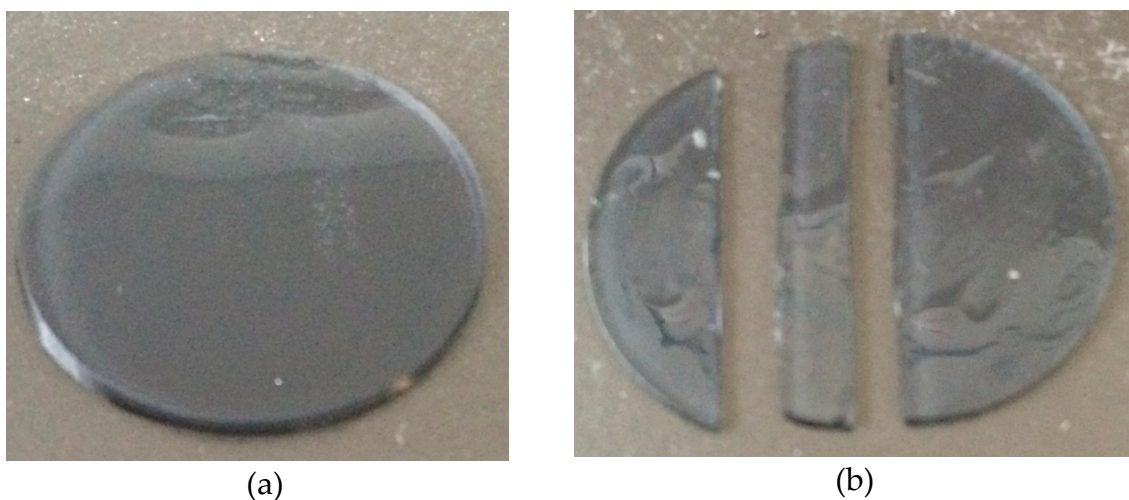
Figure 1. Image of an H77p0-clear hydrogel sample (77% water-content (w-c) hydrogel) before (a) and after (b) being cut into a strip.
