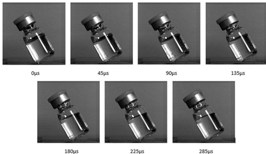
Figure 5. Cavitation time-lapse where bubbles flash across the entire fluid volume.
