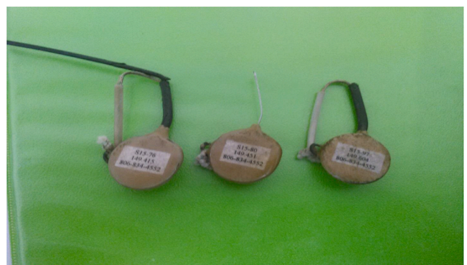
Fig. 4. VHF radio collars recovered from quail mortalities showing evidence of likely avian predation (Damaged collars appear on right, with an undamaged collar on left as reference).
