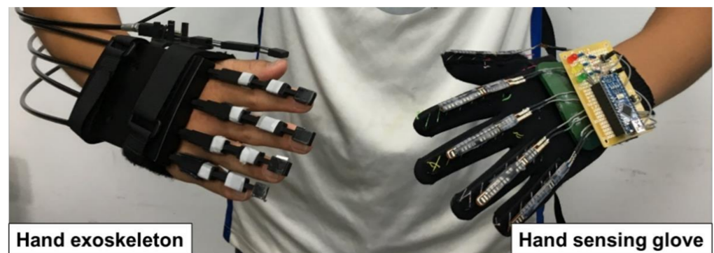
Figure 1. Framework of the bilateral hand practice, including a hand exoskeleton and a hand-sensing glove.
