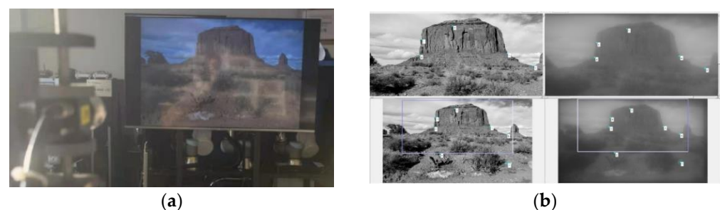
Figure 8. The key procedure constructing manual registering database; (a) The display-capture lab setup; (b) The interactive selection of artificial feature points in MATLAB software.
