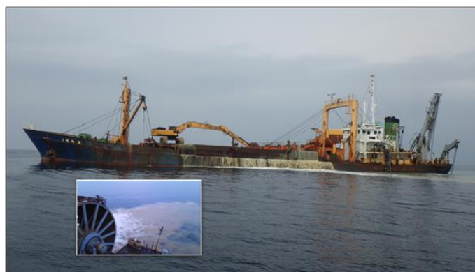
Figure 1. Photo of sediment load and dredging, i.e., sand mining activity in southern coastal waters of Korea. The designated sand mining areas are approximately 80 m deep and 100 km away from the main land of Korea (Figure 2). Overflowing of pumped bottom sand or sediment is remarkable around the ship and the spreading of overflowed sands is indicated as seen in the small photo.
