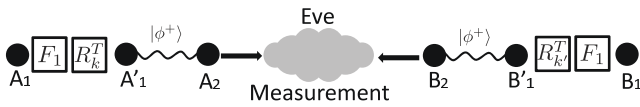
Figure 8 | Schematic that is equivalent to the EDP for n = m = 1 . While Eve accesses only the photons in modes A_2 and B_2 in the actual protocol, we pessimistically suppose that she can prepare any state in A'_1 and B'_1 for simplicity of the proof.
