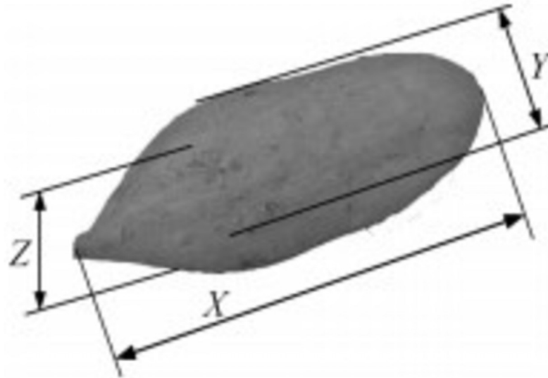
Fig 3. Characteristic dimensions of sweet potato. Calibrate the size characteristics of sweet potato.
