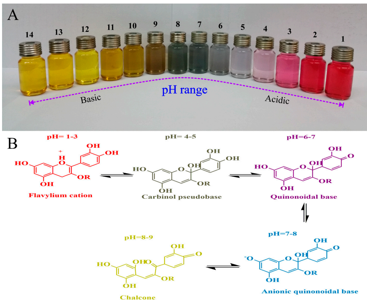
Figure 4. Solution color variations (A), and structural transformation of saffron petal anthocyanins in various buffer solutions (B), Reprinted from [42], copyright 2021, with permission from Elsevier.
