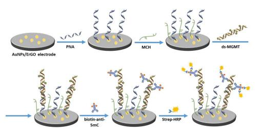
**Figure 1.** A schematic of the developed biosensor. The preparation of the AuNPs/ErGO electrode is depicted in Figure A1.
