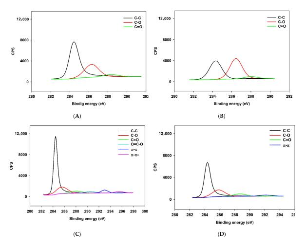
**Figure A3.** The C1s high resolution spectra of a bare electrode (**A**) and GO- (**B**), ErGO- (**C**), and TrGO- (**D**) modified electrodes.
