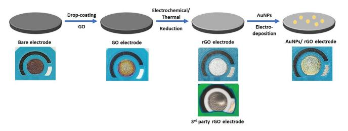
**Figure A1.** A schematic of the surface modification procedure of a screen-printed electrode (Section 2.3) and the changes to the appearance of the working electrode.
