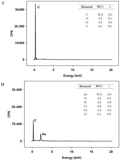
**Figure A6.** SEM images of ErGO (**A**) and ErGO/AuNPs (**B**) electrodes. EDS spectra of the ErGO (**C**) and ErGO/AuNPs (**D**) electrodes. The inset tables show the present elements, the relative concentration (Wt%) of each element, and their measurement errors ( $\sigma$ ).
