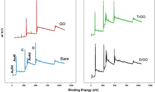
Figure 4. XPS spectra of the bare electrode and electrodes modified with GO, ErGO, and TrGO after the deposition of the AuNPs. The ErGO showed the highest At% for Au.
