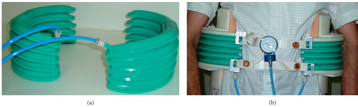
FIGURE 12: Multichamber SPA (a) and the prototype of the active brace (b).
