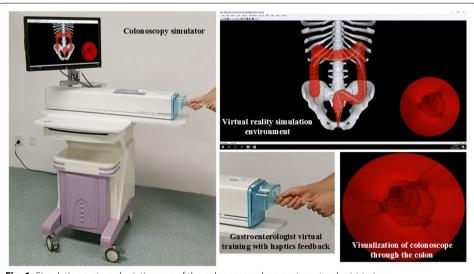
Fig. 1 Simulation system depicting use of the colonoscope by a gastroenterologist trainee
