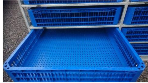
Figure 1. High-density polyethylene crates in a steel frame used to transport chickens to slaughter.
