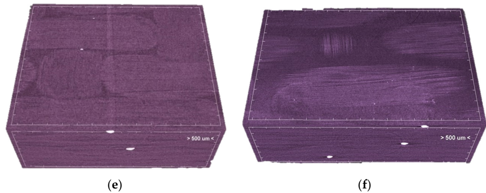
Figure 3. Internal structure of CFRP pre-exposure (a) untreated, (c) PMAA, and (e) APP; post-exposure (b) untreated, (d) PMAA, and (f) APP.
