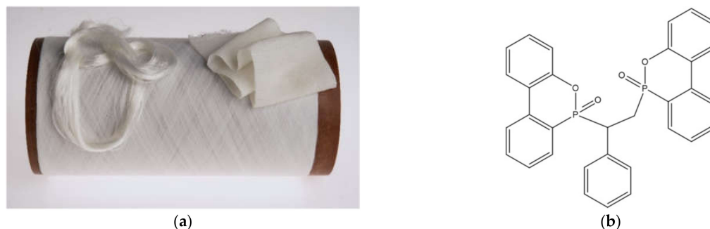
Figure 1. The flame-retardant (PA6)/bridged 9,10-dihydro-9-oxa-10-phosphaphenanthrene-10-oxide (DOPO) derivative nanocomposite filament yarns (a) and molecular structure of the flame-retardant bridged DOPO derivative (6'-(1-phenylethane-1,2-diyl)bis(dibenzo[ c,e ][1,2]-oxaphosphinine-6-oxide), PHED) (b).
